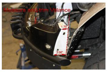
3. Measure and Cut away pinch welds at the rear of the wheels. Start at 6.75" down from mount, see picture below right, and cut down to the end of the curve in the body. Clean up any burrs and coat to protect the bare surfaces.
