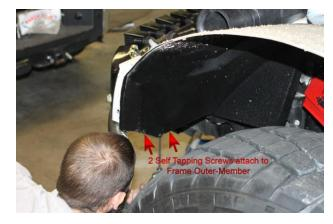
6. Find the three mounting tabs, starting from the large tab put into position and drill a 1/8" hole. Use the self tapping screw to attach to the Fender Inner Frame. Once the tab is attached drill the tabs with the 3/16" drill bit and attach the rivets with fender washers between from the inside of the Fender Inner. Continue same procedure for the Medium and Small Tabs.
