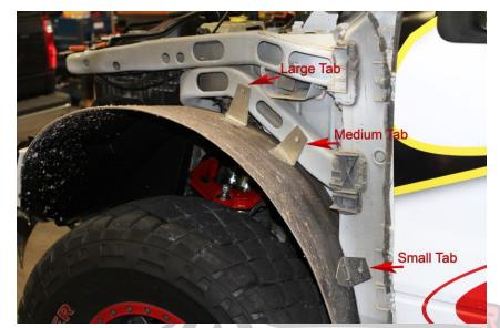
\*\*Make sure the fender is pushed into the wheel well into the pinch weld as each tab is attached.
