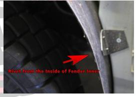
7. Once all of the tabs are installed and riveted securely, install the Boatec Fenders according to their instructions ensuring the Fender Inner is tucked under the Fender Edge. At this time there may be some trimming necessary, use care in removing material to be sure the Fenders and Liners fit together properly.
