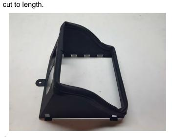
**Step 4:** Install the rubber intake support to the heat shield, and tighten.
