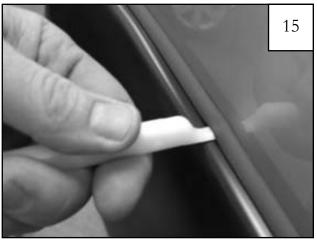
Using flat end of supplied Edge Trim Tool (ET1-0002), seat edge trim against flare by inserting straight end between edge trim and flare at one end. Next, slide around entire edge to the other end.
