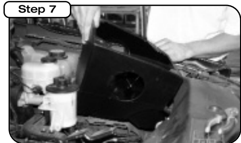
Step 7 Install housing into vehicle. With hardware provided, install M6 x1x30 screw and washer into radiator support. Install to bottom of housing, M6x1x25 screw with washers and M6 nut. With screw from step 6 install into hole with threaded insert, also in bottom of housing.
