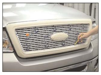
5. For mesh grilles that are black from the factory. proceed to Step 9. If the factory grille insert is not black, draw a line with the edge of the E&G grille, then remove the grille.
