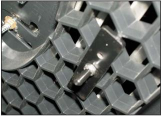
P. Reinstall the thread protectors that came installed on the grille to cover the exposed threads.
