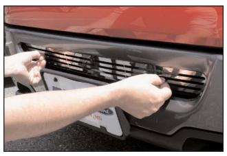
Carefully pass the lower "Q" grille through the existing opening in the metal bumper, making sure that the lower mounting brackets line up with the mounting holes in the metal bumper.
