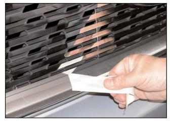
10. Remove the protective masking tape applied to the factory grille surround. Pull the tape back over itself to prevent the tape from tearing. If the grille fits tight and the tape binds, you can pull up on the grille and pull down on the factory grille frame for the added clearance needed to remove the tape.
