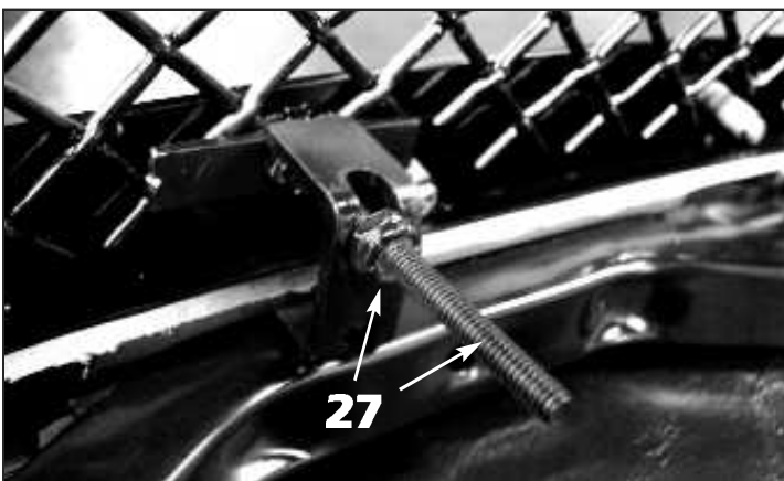
27. Paint all studs and ESNA nuts that could be visible through the mesh grille with flat or semi-gloss black paint prior to grille installation.
