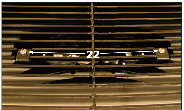
22. For customers requesting the factory emblem installation: Align the emblem assembly with the notches in the back of the billet grille. Install the mounting brackets using the supplied s.s. lock washers and s.s. #8-32 s.s. hex nuts and tighten until the emblem assembly is snug against the billet grille fins.
