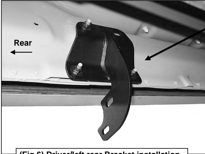
(Fig 6) Driver/left rear Bracket installation
