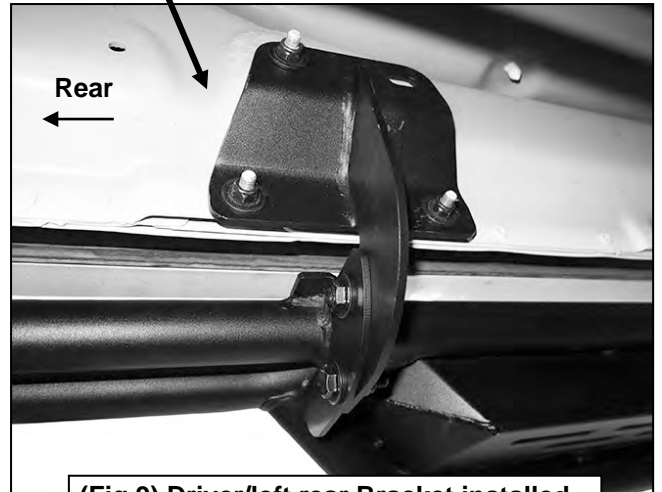
(Fig 9) Driver/left rear Bracket installed
