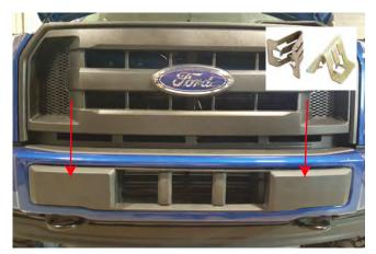
**STEP 1** // Using a panel removal tool, remove the plastic bumper insert. It is held in with several metal push clips.
