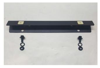
**STEP 4** // Attach the front license plate bracket to the new Barricade bumper if a front license plate is required using the (2) M6 screws, lock washers, and nuts.
