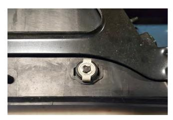
**STEP 4** // Using your factory ignition key, turn the spare tire lock clockwise and remove the spare tire lock from the factory bumper. Then install it in the new Barricade bumper.
