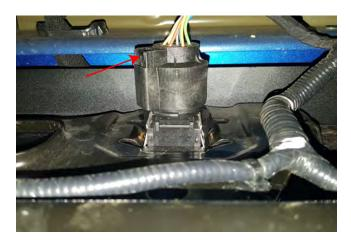
**STEP 1** // Unplug the factory license plate light harness and the trailer plug connector and pull away from the bumper.
