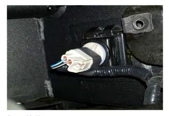
**STEP 10** // Plug the factory license plate lights harness and the trailer plug connector back in.
