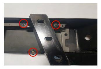
**STEP 6** // If your vehicle is equipped with a factory trailer hitch receiver, remove the (6) factory M8 bolts from the factory bumper. Install the hitch receiver to the Barricade bumper using the factory triple bolt plates through the back of the mounting tabs and then use the (6) plastic bolt holders to secure.
