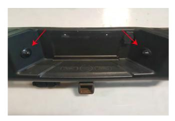
**STEP 4** // Using a flat head screw driver, push in the plastic tabs around the license plate lights, and remove it from the factory bumper. Install these in the new Barricade bumper by pushing them in place till they snap in.
