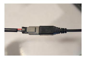
**STEP 10** // If purchased with the LED lighting option, connect the (2) LED lights into the supplied harness. Be sure to zip tie the access wiring away from any damage that could occur.
