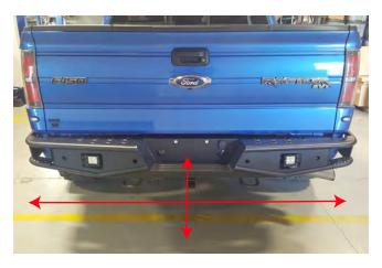
**STEP 8** // Attach the new Barricade bumper to the vehicle using the factory (6) 21mm nuts. Be sure to center the bumper, and adjust height of bumper to desired location.
