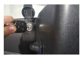
**STEP 3** // Using your factory key, turn the spare tire lock clockwise and remove the spare tire lock from the factory bumper. Then transfer it to the Barricade bumper.
