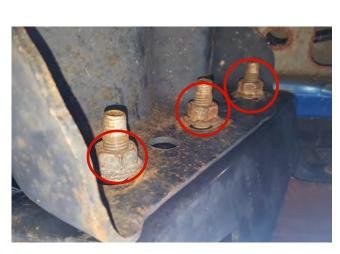
**STEP 2** // Remove the (6) 21mm nuts that hold the bumper to the frame rail. Remove bumper from vehicle.
