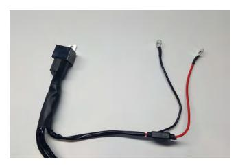
**STEP 11** // If purchased with the LED lighting option, Install the Red 12+ volt wire to the positive battery terminal. Connect the black ground wire to the negative battery terminal. Mount the fuse in a safe location away from any damage that could occur. Tuck away any extra wiring.
