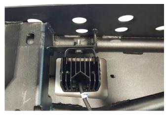
**STEP 5** // If purchased with the LED lighting option, install the LED lights using the hardware provided in the light packaging. If choosing not to use the LED lighting. The bumper will include bolt on mesh covers. Secure the cover to the bumper using the provide (2) M6 nuts and flat washer.
