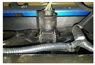
**STEP 1** // Unplug the factory license plate lights harnesses and trailer plug connector (if equipped) and pull away from the bumper.
