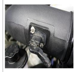
Install the silicone reducer on the throttle body and rotate down to sit in the heat shield and tighten clamps. The tube will sit on the heat shield gasket. Now install the air filter onto the end of the tube and tighten the clamp. Plug in the PCV fitting, breather hose and MAF plug. That's it!
