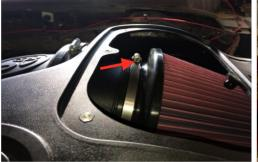
23. Insert the Air Intake Tube (B) into the Silicone Step Coupler (N) at the throttle body. Once everything is in place, tighten Hose Clamp #56 & #52 (O & P).
