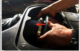
24. Reconnect the vacuum line. Push in the connector over the Quick Connect Fitting (R) until you hear it snap into place.
