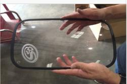
**29.** Install the Clear Lid (E) on top of the Air Box (A) and secure the lid using the six provided Truss Head Phillips Screw (M) and Sealing Washer (L). Do not over tighten.
