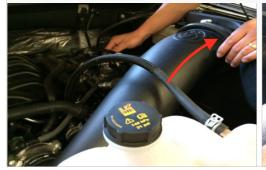
22. Tighten the Hose Clamp #88 (J) at the Air
