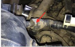
9. Lift and remove the stock air box.
