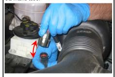
Loosen the hose clamp at the throttle body pull out and then towards the left, pulling the OE intake assembly out of the drivers side
