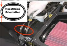
**16.** Reconnect the MAF sensor electrical connection. Check that both connectors are fully engaged.
