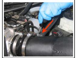
**18.** Install the S&B clear lid (R), secure with 10/24 screws (S) and sealing washers (U). Do not over tighten.
