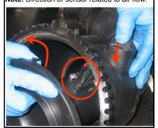
13. Install the MAF sensor into the S&B tube (C), secure with the OE screws, tighten evenly. Do not over tighten!
