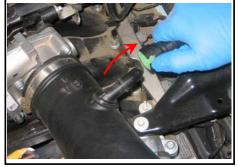
Disconnect the electrical connection for the MAF sensor at the pig tail coming from the
