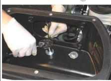
8. Place the S&B air filter (Q) inside the S&B air box (O). Offset flange is toward the front of the vehicle. Snap S&B filter adapter (J) into S&B air filter (Q) secure with #104 hose clamp (T). Use 5/16 nut driver or screwdriver.
