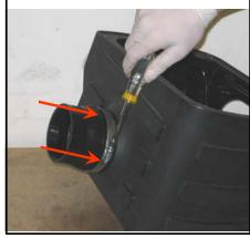
Install the S&B air box (O) and secure using the 5/16 bolts (N), fender washers (M), rubber spacers (L) and lock nuts (K) provided. See diagram below.
