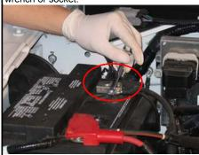
2. Disconnect the CCV line from the driver side valve cover to the OE intake tube and remove it from the vehicle
