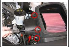
**10.** Place the Oval hump adapter (H) over filter adapter (J), do not tighten hose clamps at this step.
