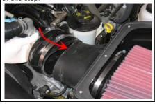
**11.** Install the step adapter (E) to S&B tube (C), secure with a #52 hose clamp (D).
