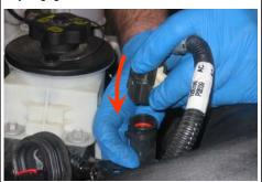
17. Install the S&B 5/8" CCV hose (A) from the valve cover to the S&B Intake tube (C), secure both ends with a #8 hose clamp (B).
