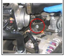
**15.** Install the S&B tube (C) into the Oval hump adapter (H) then onto the throttle body. Center the Oval hump adapter (H) over gap between tube ends and secure with #88 hose clamps (G) , then secure # 48 hose clamp (W) at throttle body.
