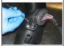
**14.** Remove the OE alternator bracket bolt just in front of the throttle body, and replace with the supplied M6 tapered allen bolt. This will allow clearance for the larger S&B tube.
