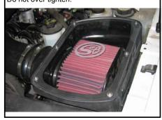
**19.** Reconnect the battery. Inspect your installation, make sure kit is properly positioned and all fasteners are secure.
