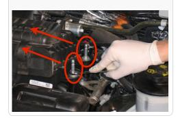
7. Unclip the wire loom from the OE air box.
