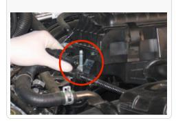
8. Pull up at the throttle body to remove the intake assembly from the vehicle.
