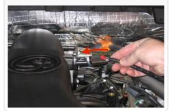
23. Install the Crank Case Vent Hose (A) at the valve cover and Intake Tube (C) on the Passenger's side. Secure both ends using the #8 Hose Clamp (B).
