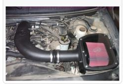
26. Reconnect the battery. Inspect your installation, make sure the kit is properly positioned and all fasteners are secure. Affix the CARB sticker near the intake kit. The installation is now complete
