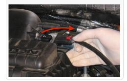
4. **IF EQUIPPED:** Disconnect the brake boost vacuum line from the air box on the Driver's side. Note: ONLY IF EQUIPPED, the S&B Intake Tube (C) must be cut at the trim line prior to installation.
