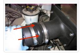
18. Install the Step Adapter (E) over the Intake Tube (C) and secure using a #60 Hose Clamp (D). **Note:** You may find it easier to install the Adapter (E) on the throttle body first then install the Intake Tube (C) in Step #21.
