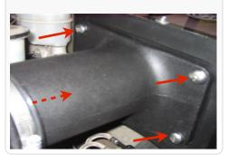
17. Place the Hump Adapter (H) and #72 Hose Clamp (G) over the Filter Adapter (J). Do not tighten at his time.
