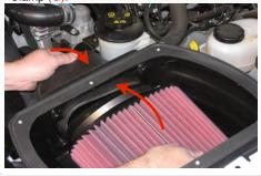
16. Secure the Filter Adapter (J) to the Air Box (O) using the 4 supplied 5/16" Phillips Head Screw (I).
