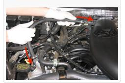
24. IF EQUIPPED: Attach the OE brake boost vacuum line to the Intake Tube (C) on the Driver's side and secure using a #8 Hose Clamp (B). Caution: Intake Tube (C) must be modified if equipped with vacuum line. See step #4
