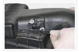
20. Install the MAF sensor into the Intake Tube (C), evenly secure using the OE screws. DO NOT OVER TIGHTEN
