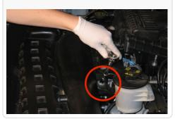
6. Remove the 4 studded bolts that secure the OE air box to the intake manifold.
