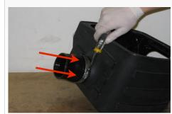
13. Place the Rubber Spacer (L) over the holes on the fender.
