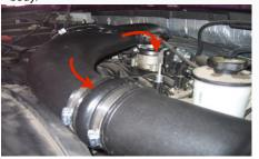
22. Reconnect the MAF sensor electrical connection.
