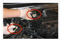
3. Disconnect the electrical connection for the MAF sensor, at the air box on the Driver's side.
