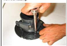
12. Assemble the MAF sensor, heat shield and the filter adapter using the two gaskets and 1/4-20 x 1" bolts provided.
