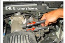
7. Pull up to release the OE air intake tube assembly from the grommets. And remove it from the vehicle
