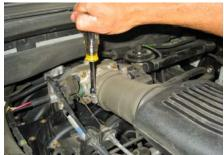
6. Disconnect the electrical connection for the MAF sensor.
