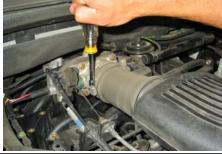
10. Release the four clips that secure the MAF sensor housing by pushing with a flat blade
