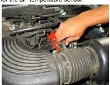
4. (a) On 4.6L Engines: Disconnect both the air bypass valve line and the crankcase vent line from the OE air intake tube.
