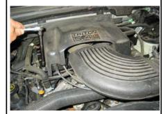
5. At the throttle body, loosen the hose clamp on the OE air tube.
