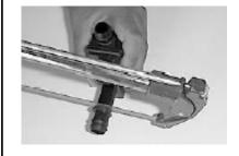
21.(b) On 5.4L Engines: Attach the provided 3/4"x6" hose to the crank case vent line and secure both the vent and idle air control lines to the S&B intake tube. Use the #8 Hose Clamps. If the OE vent line allows, you may cut the provided hose shorter as pictured below.
