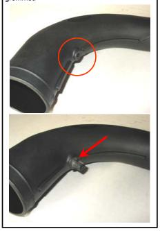
**15.** Remove the OE rubber grommets from the inner fender bracket.
