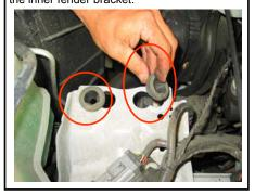
**16.** Install the speed nut clips to the inner fender bracket
