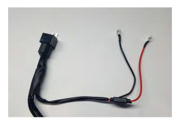
**STEP 9** // Optional LED light wiring, Install the Red 12+ volt wire to the positive battery terminal. Connect the black ground wire to the negative battery terminal. Mount the fuse in a safe location away from any damage that could occur. Tuck away any extra wiring.
