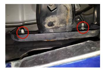
**STEP 2** // Next, loosen the upper (4) 21mm nuts holding the front bumper to the support beam of the vehicle. \*\*Note: Factory hardware will be reused.
