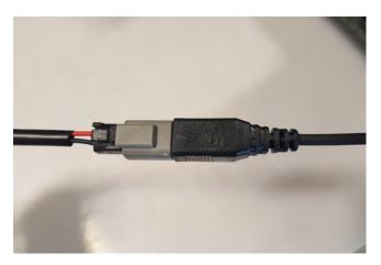
**STEP 8** // Optional LED light wiring, connect the (1) LED light bar into the supplied harness. Be sure to zip tie the access wiring away from any damage that could occur.
