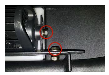
**STEP 4** // If purchased with the LED lighting option, install the LED light using the hardware provided in the light packaging. If choosing not to use the LED lighting. The bumper will include a bolt on mesh cover. Secure the cover to the bumper using (4) M8 x 20mm bolts, lock washers, and nuts.
