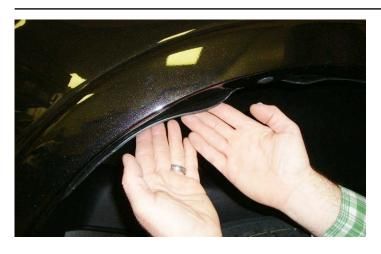
6. Tuck the remaining portion of the Wheel Well Guard behind the fender lip all the way around the fenderwell opening.
