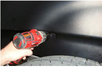
7. Push the Wheel Well Guard up until it rests against the inside of the fender well. Drill 1/8" holes at locations C and D.
