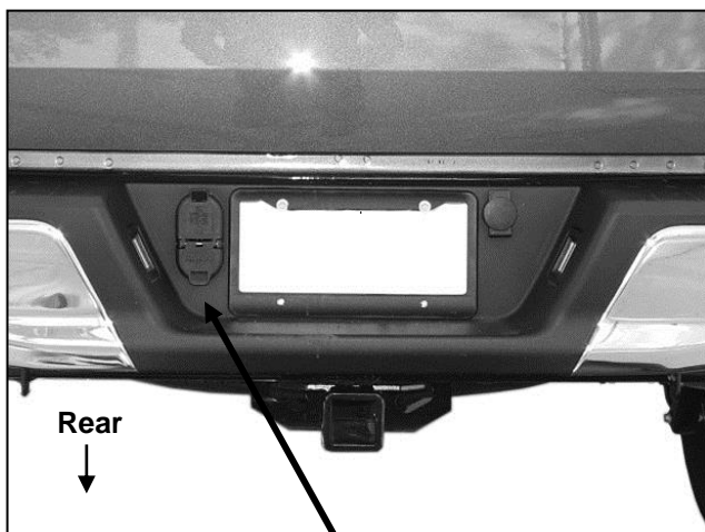
(Fig 1) Unplug and remove 7-wire trailer plug
