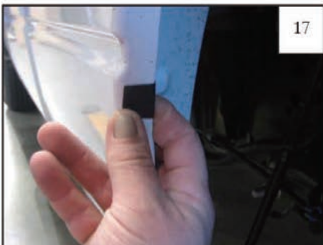
Wrap a Tab (MT1-0014) around the wheel well sheet metal, centered over each of the six marks made in Step 16.
