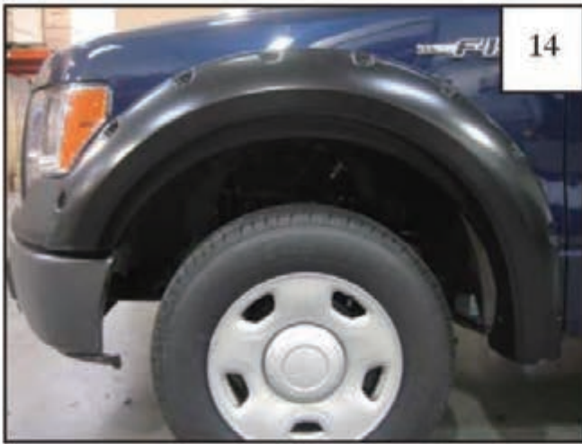
Completed front flare installation.
