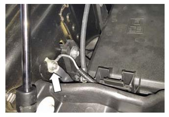
Remove the positive terminal cover from the fuse box.
