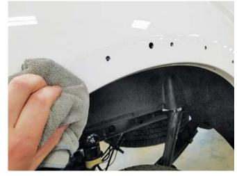
5. Set the front fender flares in place to mark the locations for the mylar pads. Apply one (1) mylar pad in the locations shown below and fold them around the lip of the wheel wells. Install one (1) J-clip around each of the mylar tabs.
