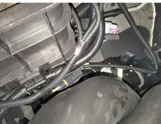
4. Remove one (1) screw with a 7 mm socket. Install the ground ring terminal from the marker light wiring harness (P/N: 1115-15N515). Re-secure the screw that was removed. Torque to 8-10 Nm.
