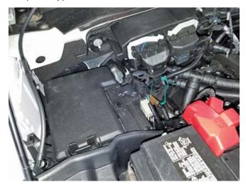
8. Install the 7.5 amp fuse that was previously removed into the fuse tap of the marker light wiring harness (P/N: 1115-15N515). Reinstall the fuse tap into the same location from which the fuse was originally removed. Trim the fuse box to allow clearance for the fuse tap lead and route the fuse tap lead through the trimmed area as shown.
