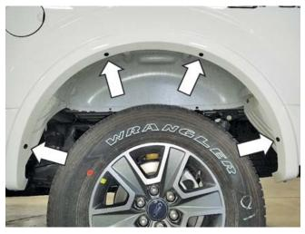
11. Firmly pull outwards on the factory rear wheel well moldings to remove them from the bed sides.
