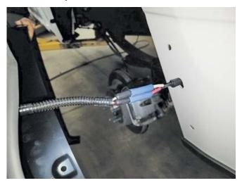
Push up and in on each flare to preload them and torque the previously installed screws to 0.9-1.1 Nm.
