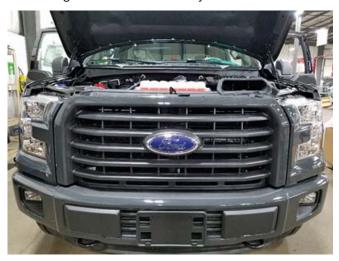
14. Use the supplied template on the last pages of the manual marked "FRONT HEADLIGHT TRIM PANEL DRILL TEMPLATE" to mark and drill an 11/16" hole in each of the front headlight trim pieces. Place the trim piece back on the vehicle to mark and drill an 11/16" hole in each of the large plastic brackets below the headlights.
