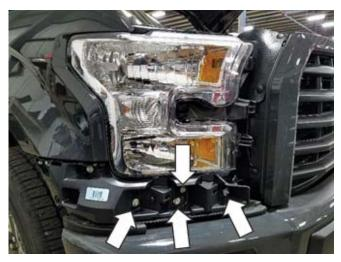
8. Remove two (2) screws with a 10 mm socket which retain the headlight. Disconnect the electrical connectors and set the headlight aside in a safe place.
