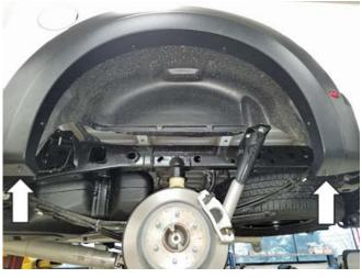
12. Use the supplied nylon trim tool and carefully slide it along the edge seals to ensure that they are fully seated.
