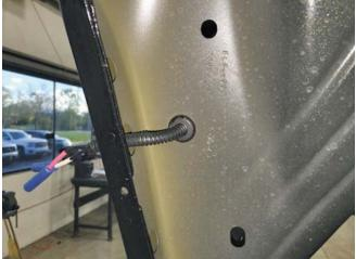
20. Secure the wire harness as shown with the edge clips (P/N: 156-00865).
