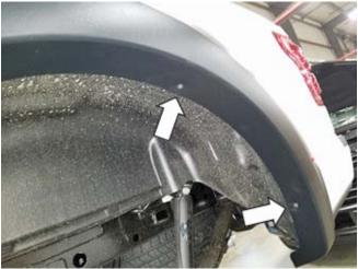
11. Install two (2) screws with a 10 mm socket that were previously removed in step 10. Torque to 0.9-1.1 Nm. **NOTE:** If the vehicle was not equipped with factory wheel lip moldings, these holes will need to be marked and drilled to utilize the No Wheel Lip Molding Hardware Kit (P/N: 1115-HWKWLM). Drill the holes to 1/4" then install the M6 J-clips (P/N: N523332) and bolts (P/N: R18020009-00).
