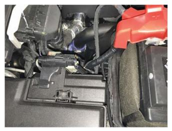
Remove one (1) nut with a 10 mm socket from the front positive terminal post. Install the positive ring terminal from the marker light wiring harness (P/N: 1115-15N515) and re-secure the 10 mm nut that was removed. Torque to 8-10 Nm.
