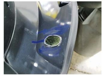
Install one (1) amber marker light assembly (P/N: 1115-AMBLTE) into each of the front marker light brackets. Remove the red backing from each piece of tape and secure the assembly to each front fender flare as shown.
