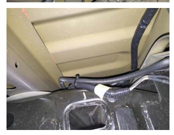
17. At the rear of the vehicle, secure the wiring harness using the provided edge clips (P/N: 156-00865).
