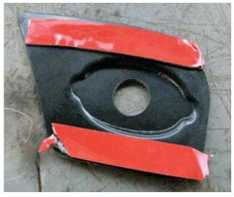
2. Wipe the back of each fender flare with the supplied adhesion promoter packet (P/N: 021200-27571) as shown.
