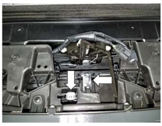
10. Remove two (2) screws from the bottom side of the factory rear wheel well moldings with a 10 mm socket. Using a non-marring trim tool, remove four (4) push pins from each of the factory rear wheel well moldings (if equipped).
