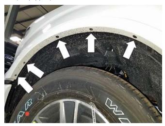
2. Remove two (2) fasteners with a 7 mm socket from the rear of each front wheel well.
