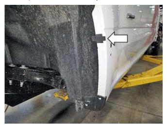
6. Set each of the front fender flares in place on the vehicle while connecting the wiring harness for each marker light. Loosely install four (4) #2 Philips head screws as shown. NOTE: Before tightening the screws, make sure the rubber edge seal is fully seated and not rolled under the flare.
