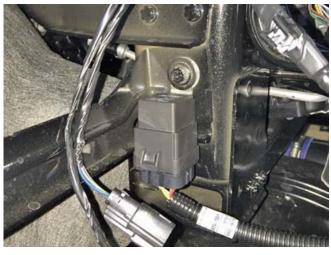
Route the two (2) ring terminals and the fuse tap up along the factory harness that passes over the windshield solvent bottle as shown. Secure with the included zip ties (P/N: CTUV740).
