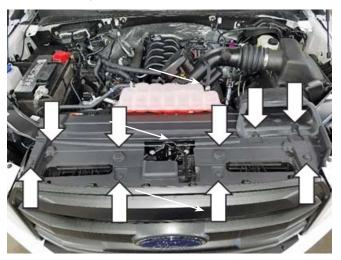
7. Remove one (1) pushpin and six (6) screws with a 10 mm socket. Remove one (1) screw with an 8 mm socket. Disengage the retaining tabs and remove the large plastic bracket below the passenger side headlight.
