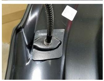
4. Install one (1) red marker light assembly (P/N: 1115-REDLTE) into each of the rear marker light brackets. Remove the red backing from each piece of tape and secure the assembly to each rear fender flare as shown.
