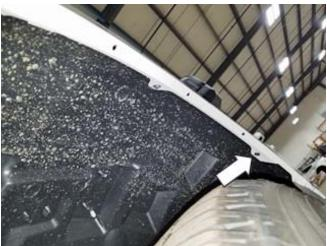
Install one (1) front fender flare inner retaining bracket on each side of the vehicle using the three (3) screws that were removed in the previous step. Torque to 0.9-1.1 Nm.
