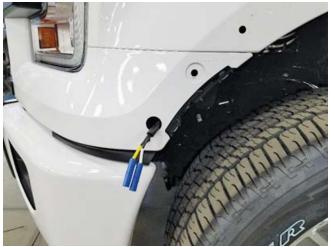
16. Continue routing the harness down along the driver side frame rail and secure with the provided zip ties (P/N: CTUV740) and edge clips (P/N: 156-00865) as shown.
