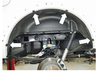
9. Set each of the rear fender flares in place on the vehicle while connecting the wiring harness for each marker light. Loosely install four (4) #2 Philips head screws as shown. NOTE: Before tightening the screws, make sure the rubber edge seal is fully seated and not rolled under the flare.
