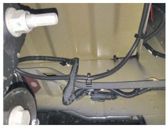
18. Use the supplied template on the last pages of the manual marked "REAR WHEEL WELL LINER DRILL TEMPLATE" to mark and drill an 11/16" hole in each of the rear wheel liners.
