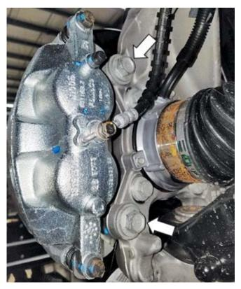
Remove the fasteners that retain the front wheel speed sensor brackets and then unclip the front wheel sensor wires from the retainers.
