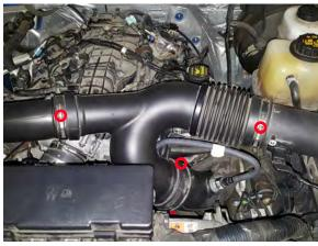
**Step 1:** Begin by using an 8mm socket and disconnecting the (3) hose clamps around the intake tube.
