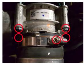
Step 2: Using a 8mm socket, loosen the intake tube connected to the throttle body. Move intake tube away from the throttle body. Next loosen and remove the (4) throttle body bolts.
