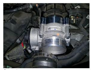
**Step 4:**Using a 10mm socket, install the throttle body spacer between the intake manifold and the throttle body using the (4) M6x70mm bolts, and washers.
