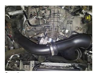
**Step 6:**Reinstall the upper intake using a 8mm socket. Installation is now complete.
