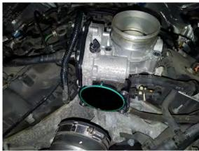
**Step 3:** Remove the throttle body from the intake manifold. \*\*Note Factory throttle body bolts will not be reused.
