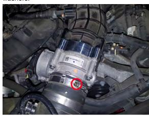
**Step 5:** Reinstall the lower intake tube to the throttle body using an 8mm socket.
