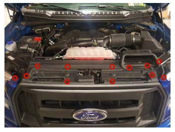
**Step 1\\**Using a panel removal tool, remove the (12) push clips holding the plastic radiator cover to the grille.
