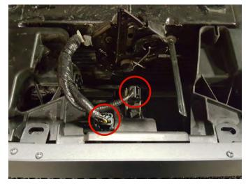
**Step 3\\**Unplug the (2) wire connections by the hood latch.
