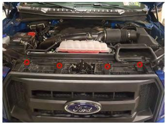
**Step 2\\**Remove the (4) 8mm bolts holding the top of the grille to the radiator support.
