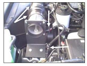
**9.** Reconnect the **MAF** sensor wiring harness to the sensor, and to the main engine wiring harness. Install the urethane hump hose (#4) onto the **MAF** sensor, with two #60 hose clamps (#13). Tighten only the clamp on the sensor.
