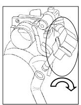
**14.** <u>**4.6L engines:**</u> Rotate the *IABV* inlet tube 90 degrees to provide clearance for the 3/4 x 12" Lhose (#7).
