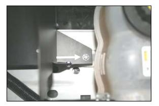
**12.** Align the hole in the **CAD** with the hole in the factory coolant reservoir mount. Insert one M6-1x25 hex bolt (#18) and 1/4" flat washer (#13) through the hole in the **CAD**, through the coolant reservoir mount, and into the speed nut below it.
