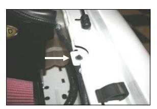
17. Slip the black plastic hose mount (#20) over the radiator overflow hose. Next, place one ½" flat washer (#13) over the hole on the inner drivers side fender. Slide the hose mount prongs thru the fender and thru the washer.
