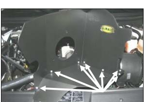
**6.** Insert three  $\frac{1}{4}$ -20 x 7/8" bolts (#12), and  $\frac{1}{4}$ " flat washers (#13) through the CAD. Place one bushing (#14) at each hole between the CAD and the filter adapter (#5). Next, secure the assembly using three 1/4" flat washers (#13), and 1/4-20 locknuts (#15).
