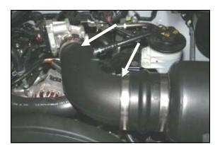
15. Install the reducer coupler (#7) onto the Airaid Intake Tube (#4) using one #48 hose clamp (#23) on the small end of the coupler, and one #52 hose clamp (#24) on the big end. Slide the tube into the hump hose first, and then over the throttle body. Adjust for fit, and tighten the clamps. Reconnect the factory breather hose.
