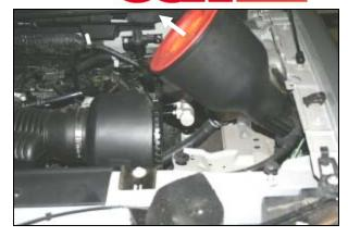
2. Remove the factory air filter and airbox from the vehicle. Pull straight up on the airbox, to release it from the grommets, and then remove the airbox inlet from the drivers side fender.
