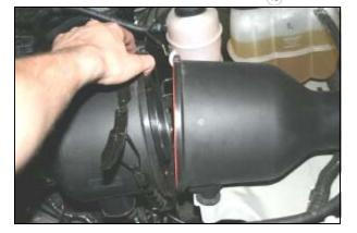
1. Disconnect the negative battery cable. Unclip the factory airbox from the factory Mass Air Flow (MAF) sensor housing.
