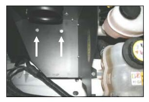
13. Insert two  $\frac{1}{4}$  - 20 x 7/8" bolts (#12) and  $\frac{1}{4}$ " flat washers (#13) through the holes in the **CAD** and thru the grommets. On the underside of the factory airbox mounting plate, align the long/narrow bracket (#19), two  $\frac{1}{4}$ " flat washers (#13), and two  $\frac{1}{4}$  - 20 locknuts (#15) with the  $\frac{1}{4}$ -20 x 7/8" bolts. Tighten the assembly securely.
