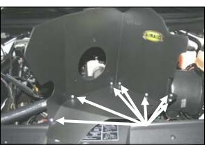
5. Assemble the Airaid Cool Air Dam (CAD) panels (#2, #3) using seven 6-32 x 5/16" screws (#9), #6 flat
