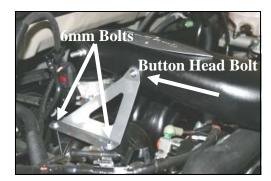
**14.** Install the two brackets (#7, #8) from the Airaid Intake tube onto the intake manifold using two  $\frac{1}{4}$  -20 x  $\frac{1}{2}$ " button head bolts (#14), and  $\frac{1}{4}$ " flat washers (#15) on the tube, and four 6mm bolts (#16), and  $\frac{1}{4}$ " flat washers (#15) on the bottom. Leave the button head bolts loose for now.
