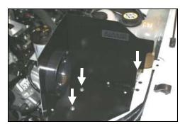
12. Install the CAD into the vehicle with one 6mm bolt (#16) and 1/4" flat washer (#15) through the panel, through the coolant reservoir mount and into the speed nut below it. Using two 6mm bolts (#16) two ½" flat washers (#15), two ½" lock washers (#17), and two M6 hex nuts (#18), insert the two bolts thru the CAD, thru the grommets, and thru the long/narrow bracket (#19). Use the line drawing above for reference.
