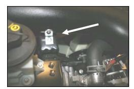
16. Install the L-shaped bracket (#25) using one  $\frac{1}{4}$ -20 x  $\frac{1}{2}$ " button head bolt (#14) and  $\frac{1}{4}$ " flat washer (#15) thru the oval slot into the backside of the tube. Next, install one 6mm bolt (#16) and  $\frac{1}{4}$ " flat washer (#15) thru the round hole into the factory bracket. Tighten the hose clamps on the hump hose. Some adjustment of the factory bracket may be necessary for a proper fit, see step #17.
