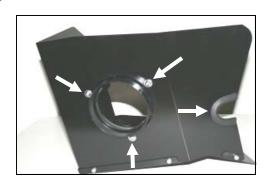
**10.** Install the air filter adapter (#2) into the **CAD** using three  $\frac{1}{4}$  - 20 x  $\frac{1}{2}$ " button head bolts (#14) and  $\frac{1}{4}$ " flat washers (#15). Next, install the 4" rubber trim (#23), as shown.
