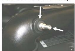
**7.** Install the rubber grommet (#20) into the Airaid Intake Tube, and then install the aluminum fitting (#21) into the grommet, tapered end first.
