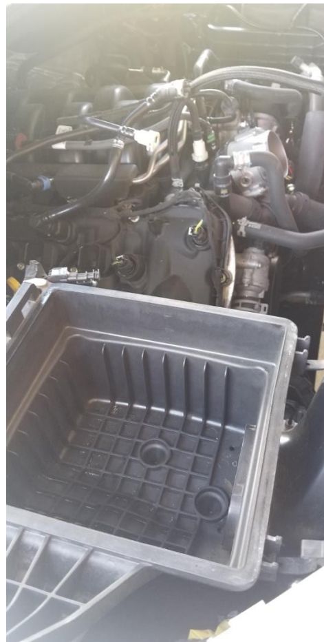
Air Filter Removed.
