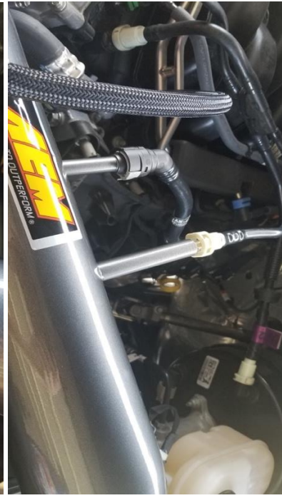
Two Hoses on the New Air Intake
