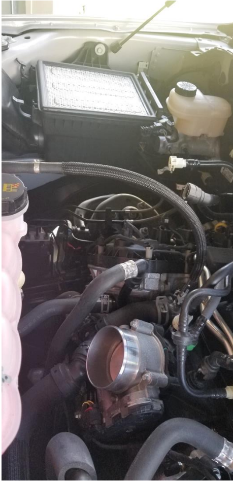
Intake Tube Removed.
