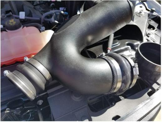
12. Slide the #68 and #64 clamp coupler onto the filter adaptor. The #68 clamp will be touching closest to the air
