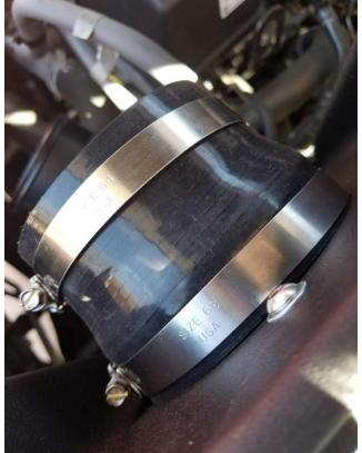
13. Connect the intake tube onto the factory turbo then into the air box coupler. You have to rotate and wiggle the tube until proper alignment is achieved. Once everything is aligned tighten all 6 hose clamps.
