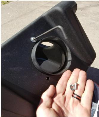
5. Insert the grommet and spacer into the side of the Airaid
