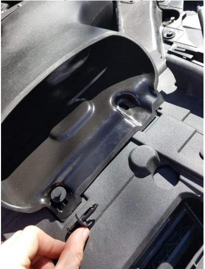
10. Secure the box to the inner fender using the 8mm bolt previously removed from existing air box (refer to set #3)
