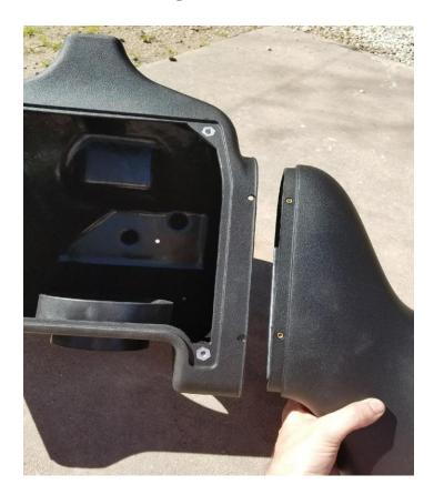
7. Once the scoop has been snapped into place use the provided two sets of 8-32 button head screws, lock washers, flat washers to secure the scoop in place.
