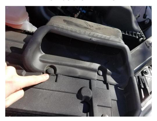
3. Remove the fender bolt on the right side of the air box assembly. Then carefully remove the entire air box from the vehicle.
