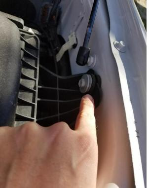
4. Mount the filter adapter on the inside of the Airaid box using the provided 3 sets of ¼-20 button head screws and washers.
