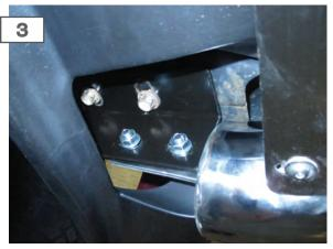
Loosely attach bar brackets to the frame rails. Mount the Bull Bar to the frame brackets securely. Then finish torqueing brackets to the frame rails.
