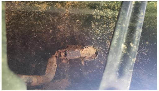
2. Disconnect both wiring plugs for license plate lights. Also, disconnect trailer plug. They have side tab you push and pull them free.
