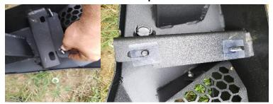
5. Install bumper to HD Towing package using 4 10mm nylon lock nuts using a 17mm socket. **Do not tighten yet.**
