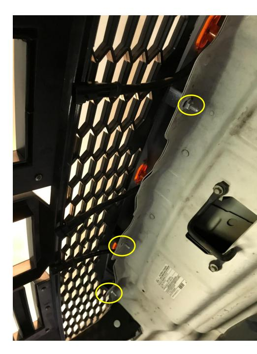
**Step 9.** Install the Bottom 6 T25 Torx bolts **Step 10.** Tighten the 6 10mm nuts on the top bolts
