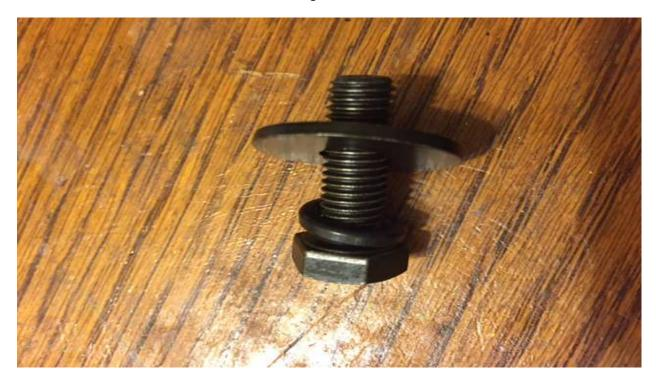
4. Install above screws to the bottom of the sidebars with brackets following the curve of the sidebars with 13mm socket (leave loose for adjustments).
