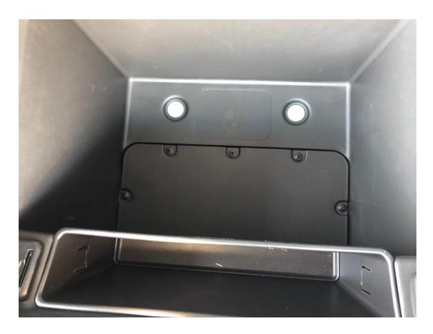
5. Open the lock vault. Place the lock vault in the empty console. Line up holes in the lock vault with threaded holes in the bottom of the console.
