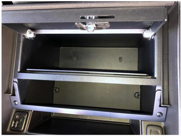
6. Use 10mm socket and ratchet to tighten provided hardware.
