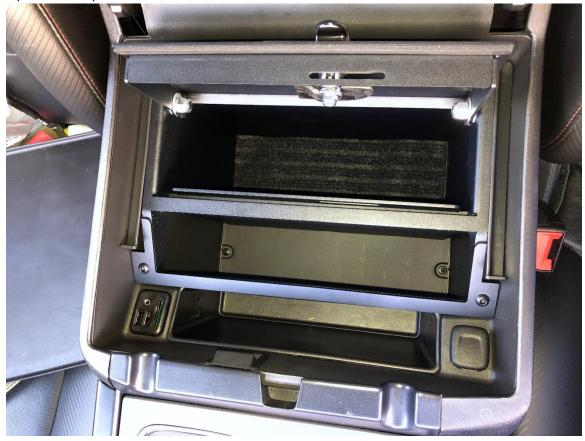
8. Ensure lock vault is securely fastened inside console. Retain file hanging capabilities. Set code according to instructions provided with lock vault.
