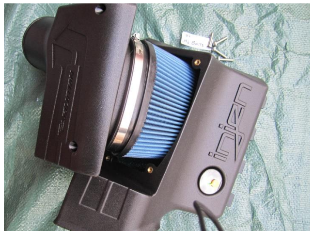
Assemble air box cover by mounting air filter, bolting to air box, using a long Phillips Screw Driver and the supplied 4 washers/seals and 4 M6 bolts:
