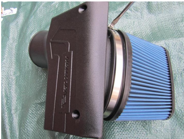
Assemble air box cover by mounting air filter, bolting to air box, using a long Phillips Screw Driver and the supplied 4 washers/seals and 4 M6 bolts:
