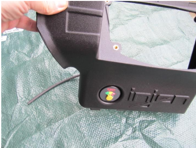
Assemble air box cover by mounting air filter, bolting to air box, using a long Phillips Screw Driver and the supplied 4 washers/seals and 4 M6 bolts:
