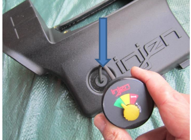
Insert air meter with vacuum hose into air box cover through grommet.
