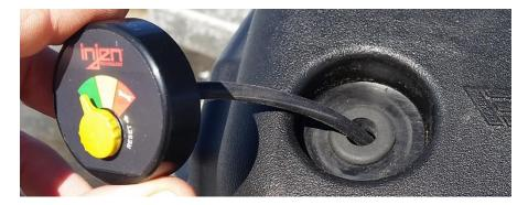
22. Drill a (5/32")hole into the top of the filter, staying at least 1" in from the edge of the filter, I drilled the hole in the small circle under the Injen logo.
