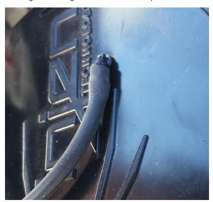
25. Attach the cover or "plenum" onto the Injen Air Box using the (4) 6x20 screws and rubber washers, you will need to use a Phillips screwdriver.
