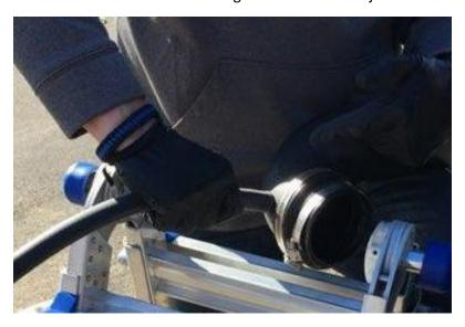
31. Attach the straight end of the Injen Air Tube with the 4"x4" hump hose connector to the Injen Air Box and tighten the band clamp using an 8mm nut driver.
