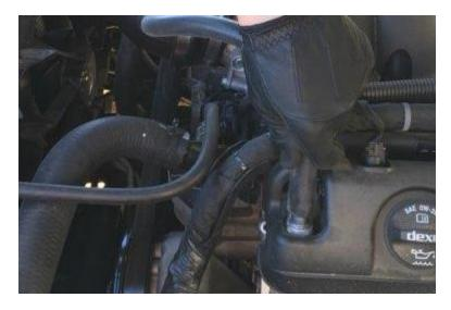
34. Insert the MAF Sensor into the Injen Air Tube.
