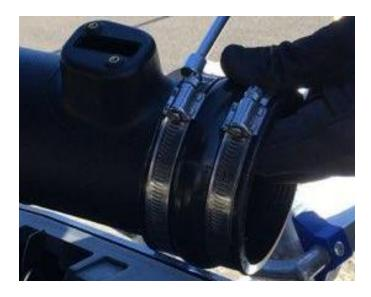
28. Attach the 4" side of the step hose connector onto the bent end of the Injen Air Tube, and tighten the band clamp using an 8mm nut driver.
