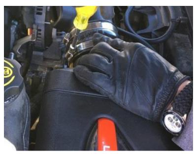
32. Attach the bent end of the Injen Air Tube with the 3.5"x4" step hose connector to the engine's Throttle Body and tighten the band clamp using an 8mm nut driver.
