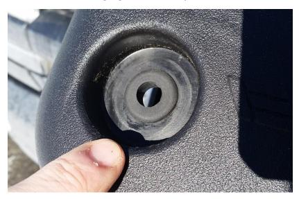
21. Run the vacuum line through the hole in the rubber grommet and install the filter monitor gauge into the Injen Air Box.
