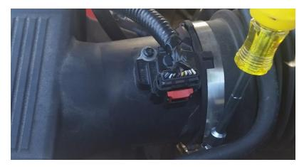
2. Using an 8mm nut driver, loosen the band clamp on the Throttle Body.
