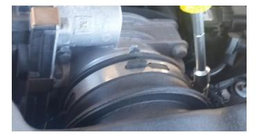
3. Disconnect both vacuum lines from the Factory Air Duct by firmly pressing the buttons to release the clamps.
