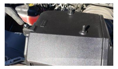
18. Attach the filter to the cover or "plenum" of the Injen Air Box and tighten the band clamp using an 8mm nut driver.
