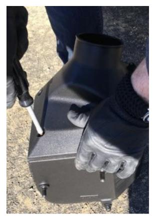
26. Install the assembled Injen Air Box onto the air box mounting plate of your vehicle by lowering it into place at an angle to clear the support bar, then align the mounting feet into the rubber grommets and push down firmly to ensure proper seating of the Injen Air Box.
