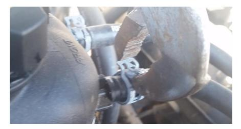
$8. \quad \text{Remove the hoses from the antifreeze overflow tank and relocate them out of the way.} \\$
