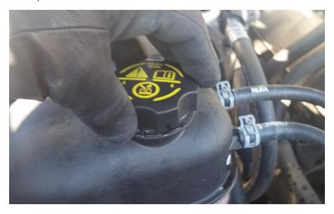
7. Using pliers squeeze the hose clamps on the hose lines on the antifreeze overflow tank and slide the clamps back on the hoses.
