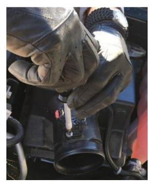
11. Remove the MAF Sensor and relocate it out of the way.
