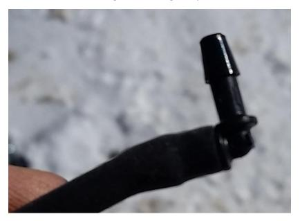
24. Insert the end of the 90deg elbow fitting into the drilled hole on top of the filter.
