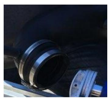
$29. \ Attach\ the\ 8.5"\ rubber\ vacuum\ hose\ onto\ the\ fitting\ nearest\ to\ the\ middle\ of\ the\ Injen\ Air\ Tube.$
