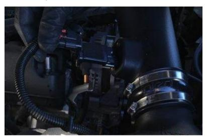
35. Attach the MAF Sensor to the Injen Air Tube using (2) M4 button head screws and an Allen Key or Hex Driver.
