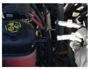
9. At the base of the Factory Air Box, engine side, remove the MAF Sensor wire tie down by gripping the tie down with pliers and pulling straight up.
