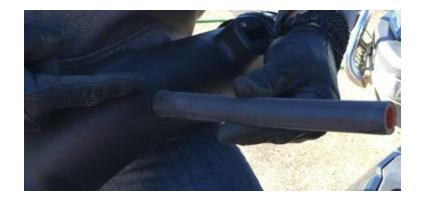
30. Attach the 14.5" rubber vacuum hose onto the fitting at the end of the Injen Air Tube.
