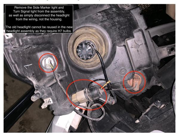
4. Remove the Factory Headlight assembly
