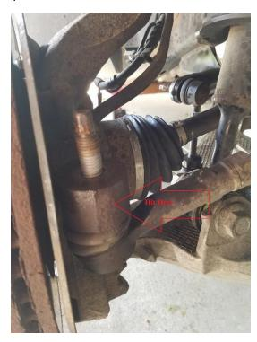
**5.** Using 12mm 12 pt socket and extension remove the 6 bolts holding the cv shaft to the differential flange.
