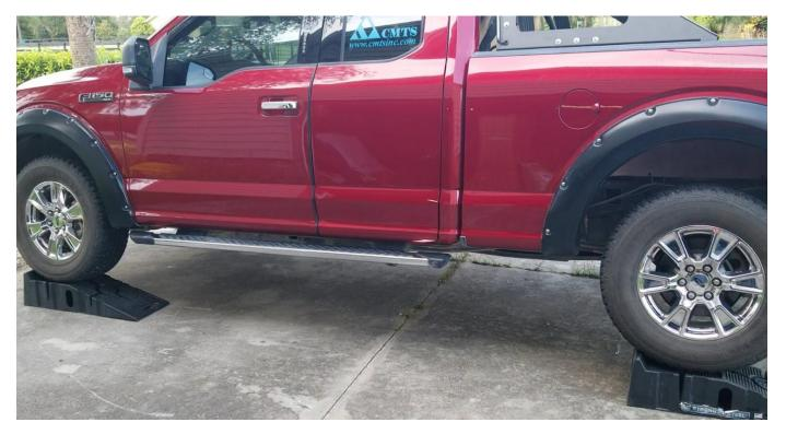
• Place one side of your truck on ramp or jack stands. Insure you're truck in level and the parking break is set. Also chock the rear tire of the other side of the truck for safety.
