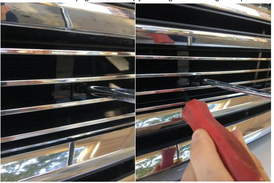
4. Check the alignment of the grille section and make sure it is centered in the opening. If everything appears to be aligned correctly, tighten the screws down until the billet grille is making contact with the vertical pieces on the factory grille and not able to move. Do not overtighten.
