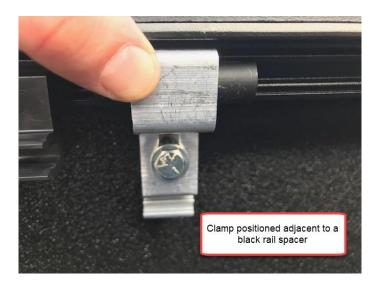
Warning! <u>Do not</u> overtighten the clamps. Also, occasionally check the clamps to ensure they remain tight.
