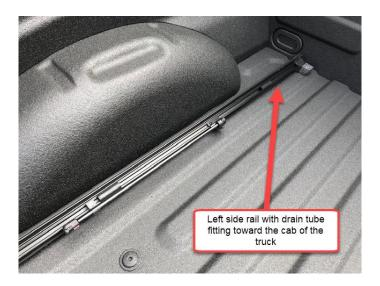
2. **Attach the side mounting rails.** Temporarily remove the proprods from the j-clips, so you can begin securing the clamps. Position the top edge of the rails level with the top edge of the truck bed.
