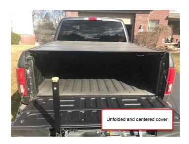
5. **Prepare to attach the cover.** Begin slowly folding the cover up by releasing each of the three release cables, being certain not to disturb the position of the cover.
