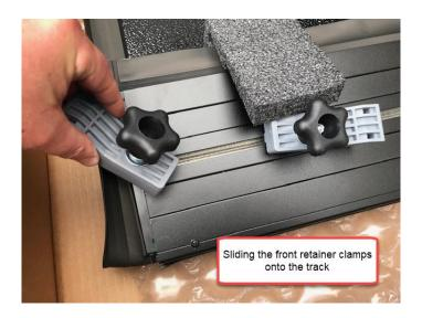
Position one on each side. Carefully place the tonneau cover onto the mounting rails with the small panel toward the cab of the truck, covering the bulkhead.
