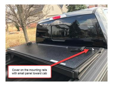
4. **Unfold and adjust the cover.** Slowly unfold each panel of the cover and position it so it is center side to side and front to back on the truck bed. Make certain you can latch the rear most section of the cover on both sides, which will indicate the cover is positioned correctly.
