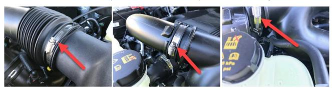
4. Locate and unlatch the two air box retaining clips on the factory filter and remove it, as well as the factory filter.
