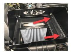
13. Install the Whipple air tube to the engine. Begin by setting the inlet side through the air box and then install the other ends to the factory air tubes. Tighten the clamps to secure the Whipple air tube to the factory tubes.
