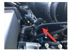
2. Carefully detach the coolant hose from the clip on the factory air tube.
