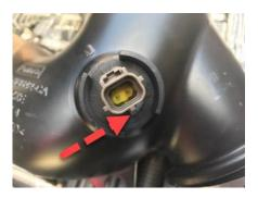
6. Install the provided IAT sensor grommet (cone side down) into the Whipple air tube.
