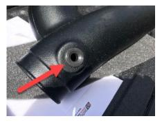
7. Gently and slowly push the IAT sensor onto the Whipple air tube. Be sure to stop once the tab on the sensor reaches the grommet on the air tube.
