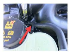
3. Locate the three clamps on the factory air tube. Loosen each and remove the air tube from the engine.
