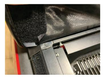
Slide the Tonneau cover into the rails at the front of the bed. The plastic portion slides into the rail on either side. Use the phillips screw to secure the tonneau cover to the rails.
