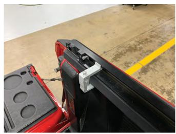
**Step 1 \\** Place the rails on the vehicle. Velcro side out with the latch portion of the rail facing the rear of the vehicle.
