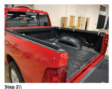
Space the rail clamps evenly over the distance of the bed of the truck. On this application (3) are used on each side. Tighten the clamps enough so that they are secure but leave them loose enough that you can still slightly move the rails. \*\*Note: For Vehicles with utility rails see note at end of install.
